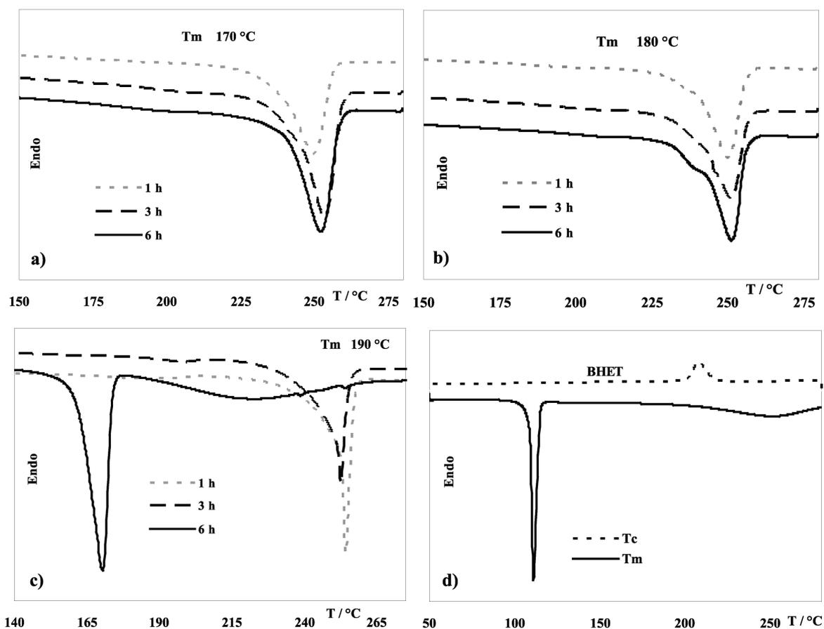
Fig. 3 – Melting temperatures ( $T_m$ ) of PET oligomers recorded after 1, 3 and 6 h at a) 170 °C, b) 180 °C, c) 190 °C and d) melting and crystallization ( $T_c$ ) temperatures of extracted monomer BHET
