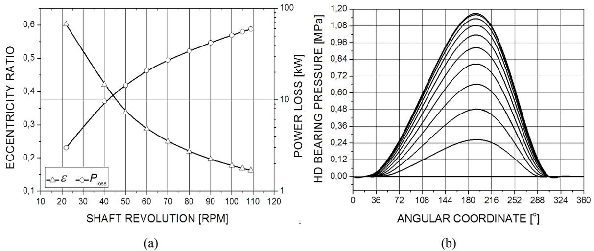
**Fig. 3** Calculated relationship between significant parameters of the stern tube white metal bearing in steady state condition with constant radial load of 1325 kN at various shaft revolutions: (a) power loss versus eccentricity ratio, (b) bearing pressure field at 109 rpm of the propeller shaft
