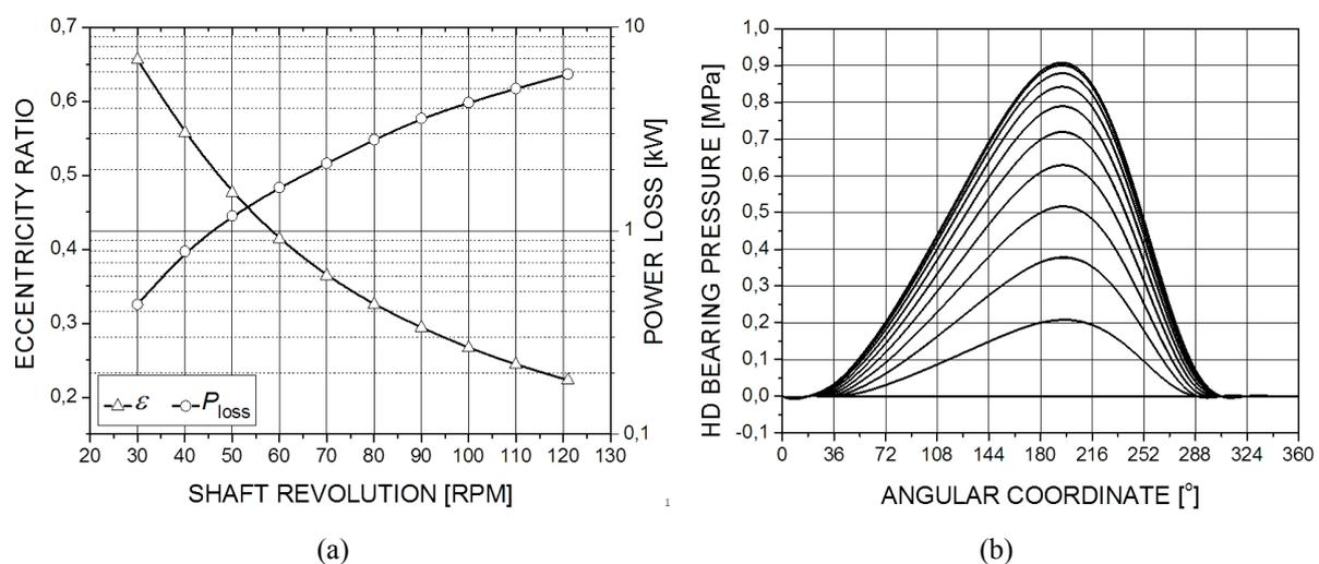
**Fig. 2** Calculated relationship between significant parameters of the stern tube white metal bearing in steady state conditions with constant radial load of 225 kN at various shaft revolutions: (a) power loss versus eccentricity ratio, (b) bearing pressure field at 121 rpm of the propeller shaft.
