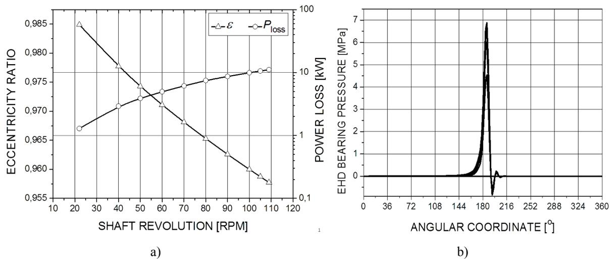
**Fig. 5** Calculated relationship between significant parameters of the stern tube with polymer bearing in steady state condition with constant radial load of 1325 kN at various shaft revolutions as follows: **(a)** power loss versus eccentricity ratio, **(b)** bearing pressure field at 109 rpm of the propeller shaft
