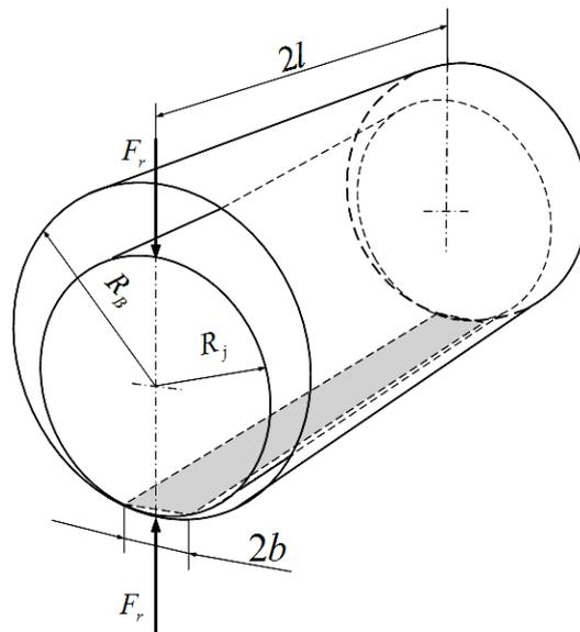
**Fig. 1** Geometry of the contact area between the journal and the bearing
