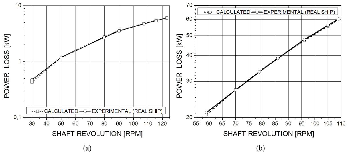
**Fig. 6** Comparison of the theoretical and experimental calculation of the power loss in aft stern tube white metal bearing at various shaft revolutions and constant bearing load: **(a)** bulk carrier of 50000 DWT, bearing load of 225 kN; **(b)** container ship of 11000 TEU, bearing load of 1325 kN.
