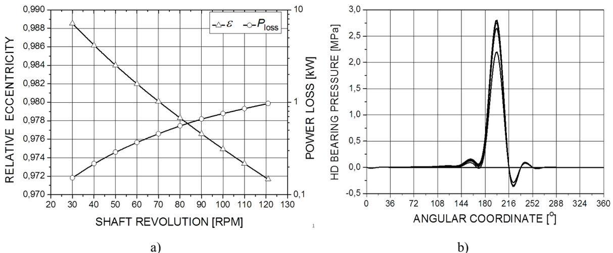
**Fig. 4** Calculated relationship between significant parameters of the stern tube with polymer bearing in steady state condition with constant radial load of 225 kN at various shaft revolutions as follows: (a) power loss versus eccentricity ratio, (b) bearing pressure field at 121 rpm of the propeller shaft.
