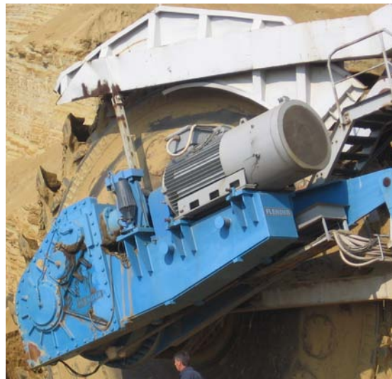
Fig. 2 Toothed gear transmission of BWE's working wheel
