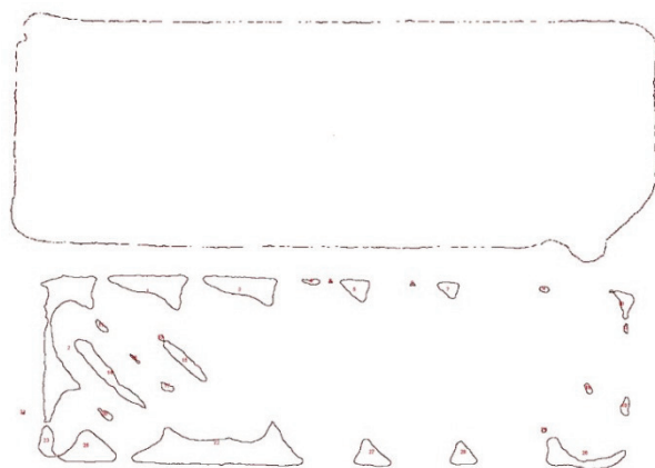
Figure 7 Outlines of the whole specimen cross-section (above) and outlines of non-filled area
