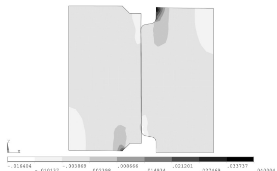
Figure 5 Calculated normal strains \epsilon_y in mineral wool core of a longitudinal joint (at load F = 1,16 kN/m)
