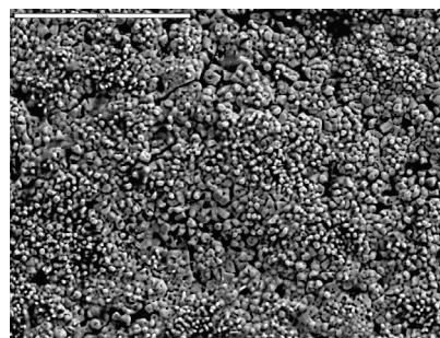
Figure 2 The microstructure of the N-155 superalloy after the creeping process (1000×); the white bar in the upper left corner indicates 50 μm.
