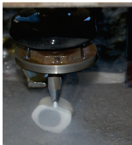
Figure 6 Cutting of femoral stem with bone cement by abrasive water jet
