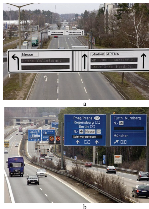
Figure 6 Dynamic route guidance system in Nuremberg, Germany.
