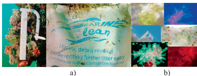
FIGURE 7 – After two months: a) all bags and test specimens were covered by a thin biofilm of different marine microorganisms, plants and animals, b) macroalgae under the microscope
