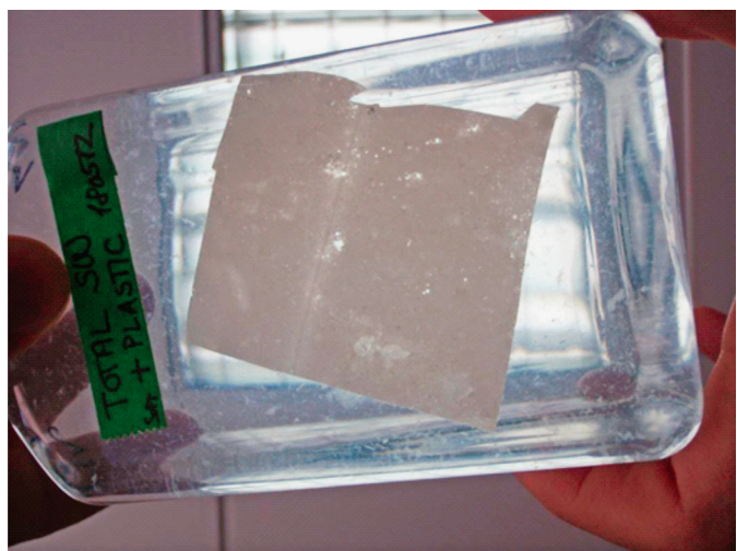
FIGURE 10 – Degradation of plastic bag in non-filtered marine water after two months
