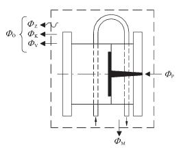
FIGURE 6 – Mould – heat exchanger:  $\Phi_{\rm p}$  – heat that thermoplastic melt brings to the mould,  $\Phi_{\rm o}$  – heat exchanged between mould and the environment,  $\Phi_{\rm z}$  – heat exchanged by radiation,  $\Phi_{\rm K}$  – heat exchanged by convection,  $\Phi_{\rm v}$  – heat exchanged by conduction,  $\Phi_{\rm M}$  – heat exchanged between mould and coolant<sup>7</sup>
