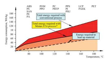
FIGURE 13 - ETA-process energy consumption<sup>18</sup>
