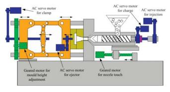
FIGURE 11 – Cross-section of all electric injection moulding machine<sup>16</sup>
