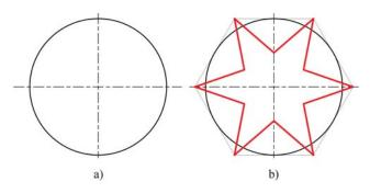
FIGURE 8 – Cross-sections of cooling channels: a - classic shape, b - shapes achievable by AM<sup>11</sup>
