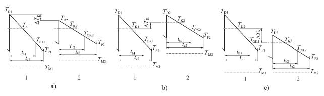
FIGURE 5 – Influence of mould material on moulded part cooling time: a - required cavity wall temperature, b - required contact temperature, c - required coolant temperature; 1 - material with lower thermal properties, 2 - material with higher thermal properties;  $T_{\rm D}$  - contact temperature (K),  $T_{\rm OK}$  - mould opening temperature (K),  $T_{\rm M}$  - coolant temperature (K),  $T_{\rm P}$  - start temperature (K),  $t_{\rm c}$  - injection moulding cycle time (s)<sup>7</sup>
