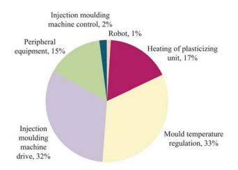
FIGURE 1 – Share of energy consumption in representative injection moulding system  $^{1} \ \ \,$
