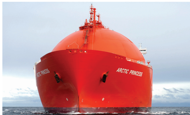
Figure 2. LNG Carrier (Moss Type) Source: http://www.hoeghling.com/shipping/fleet/Pages/Arctic-Princess.aspx
