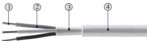
Figure 1 Product composition: 1 – Cu conductor, 2 – PVC insulation, 3 – unvulcanized tire filling and 4 – PVC sheath
