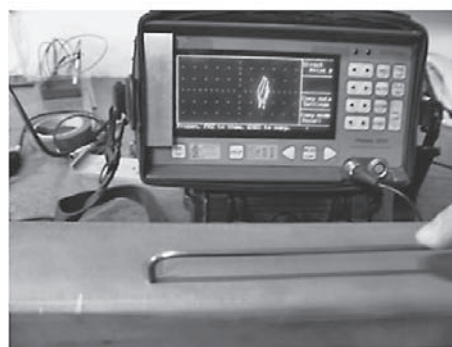
Figure 6 Rail testing using EC device Phasec 2200 (NDT Laboratory JAT in Belgrade, 2012)
