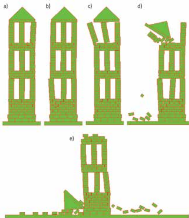
Figure 26. Stone bell tower exposed to earthquake action for peak acceleration of a_g=1.50g : a) t=6.30 s; b) t=7.32 s; c) t=11.40 s; d) t=13.44 s; e) t=18.20 s
