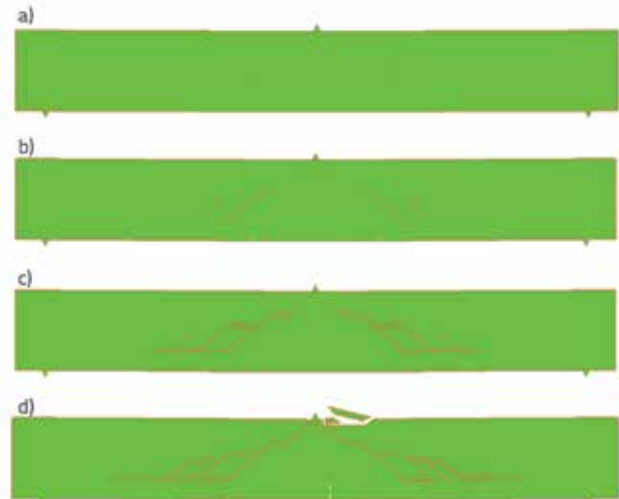
Figure 12. Structural cracks for loads: a) F=216.0 kN; b) F=259.0 kN; c) F=261.0 kN; d) F=261.1 kN
