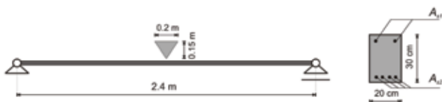
Figure 16. Geometrical properties of reinforced-concrete beam
