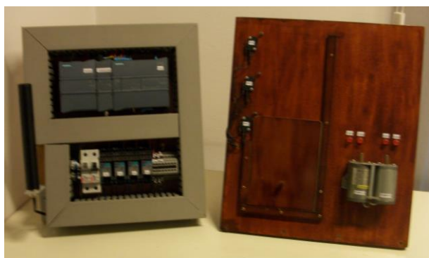
Figure 3. Pumping station prototype model
