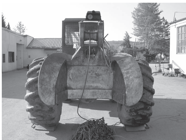
Slika 10. Zadnja daska i valjci vitla na skideru Timberjack 240C Fig 10. Rear protection plate and winch rollers on skidder Timberjack 240C
