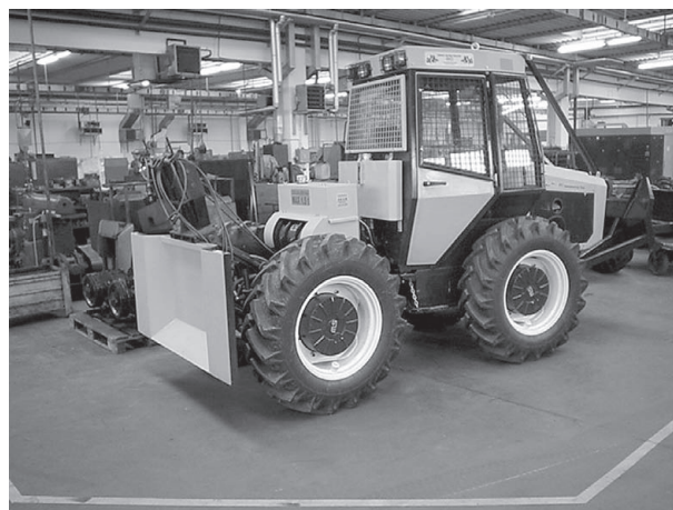
Slika 12. Nova sidrena daska Ecotrac-a 55V Fig 12. New rear anchor plate of Ecotrac 55V
