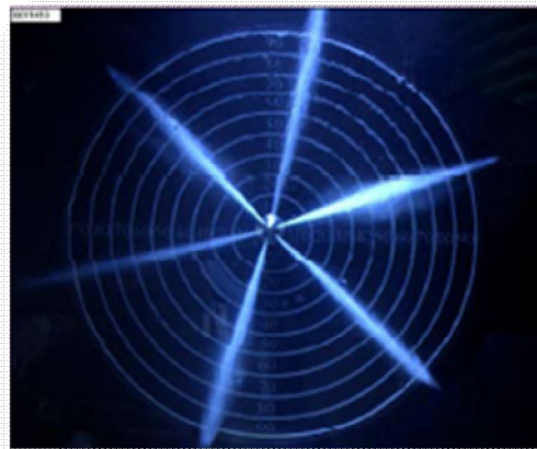
Clean injector nozzle
