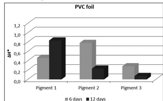
Figure 5: Hue differences of pearl luster pigments printed on PVC foil.
