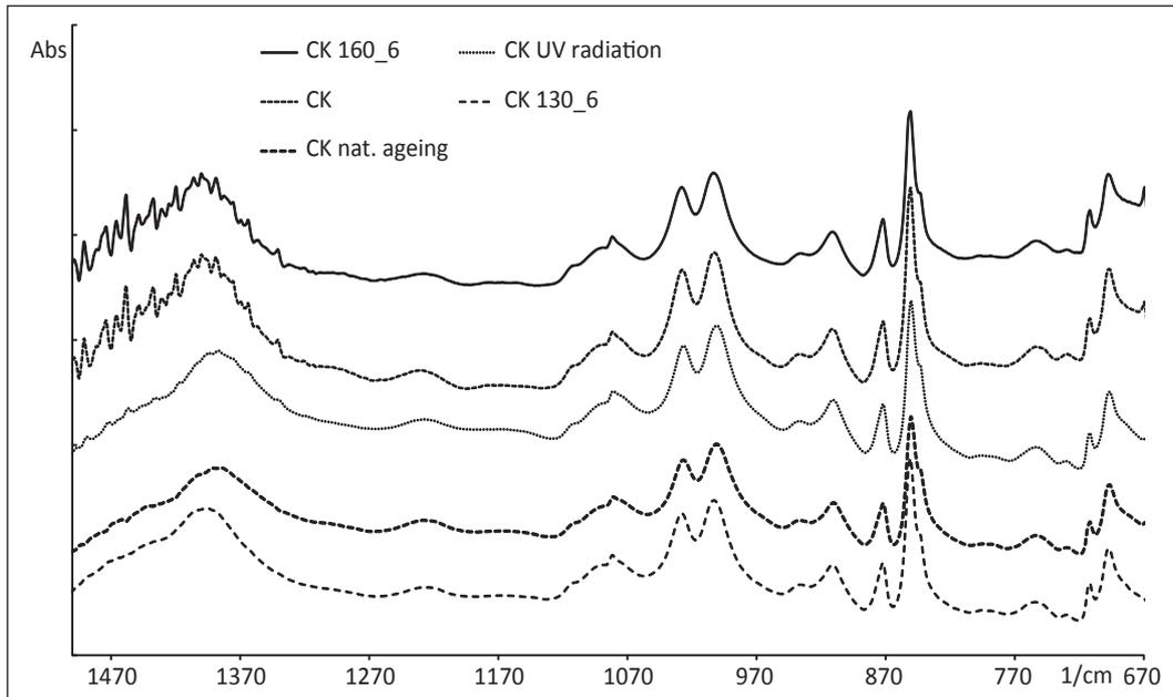
Figure 10. IR spectra of coated samples printed with Black ink before and after ageing (spectra are shifted in absorbance for clarity)
