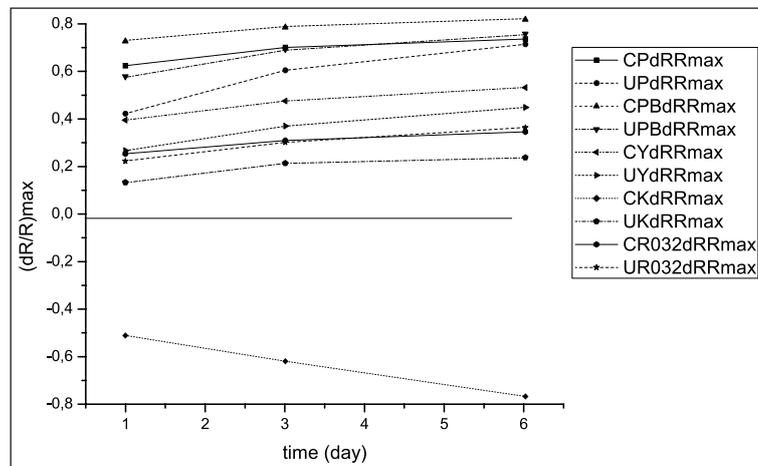
Figure 6. Maximum relative reflectance differences at specific wavelength,  $(dR/R)_{\max}$  for all measured samples after they had been exposed to heat in the oven at 160 °C for one, three and six days.
