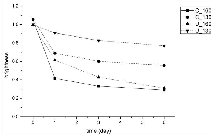
Figure 8. Dependence of paper brightness on the duration of accelerated ageing
