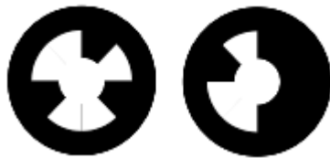
Figure 9: Circle Markers (Naimark and Foxlin, 2002)
