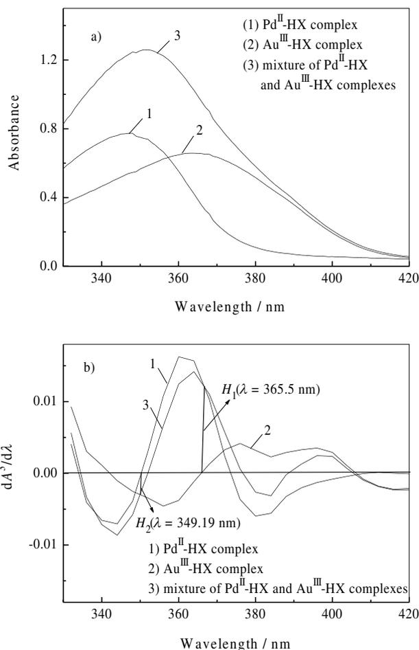
Figure 3. Zero-order (a) and third-derivative spectra (b) of Pd<sup>II</sup>-HX complexes, Au<sup>III</sup>-HX complexes and their mixture; pH = 2.5,  $c(\text{HX}) = 1.6 \times 10^{-3} \text{ mol dm}^{-3}$ ,  $c(\text{Pd}^{\text{II}} \text{ or } \text{Au}^{\text{III}}) = 4 \times 10^{-5} \text{ mol dm}^{-3}$ .
