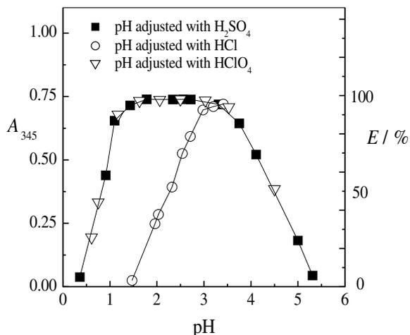
Figure 1. Dependence of Pd<sup>II</sup>-HX complex absorbance and palladium(II) extraction on the pH;  $c(\text{Pd}^{\text{II}}) = 4 \times 10^{-5} \text{ mol dm}^{-3}$ ,  $c(\text{HX}) = 1.6 \times 10^{-3} \text{ mol dm}^{-3}$ .
