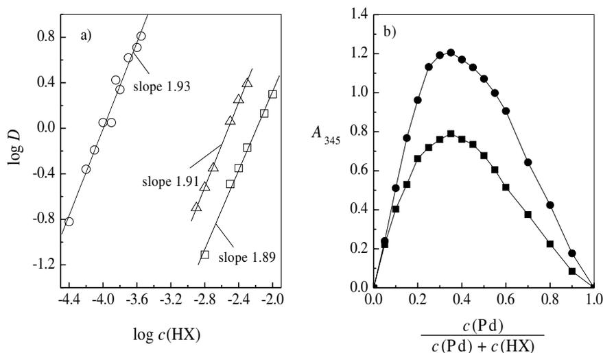
Figure 2. Determination of the composition of the extracted Pd-HX complex by slope analysis (a) and Job's method (b). a)  $c(\text{Pd}^{\text{II}}) = 4 \times 10^{-5} \text{ mol dm}^{-3}$ , pH = 2.5 (O), 0.78 ( $\Delta$ ), 0.6 ( $\square$ ); b) pH = 2.5,  $c(\text{Pd}^{\text{II}}) + c(\text{HX}) = 2.5 \times 10^{-4} \text{ mol dm}^{-3}$  ( $\blacksquare$ ),  $c(\text{Pd}^{\text{II}}) + c(\text{HX}) = 3.0 \times 10^{-4} \text{ mol dm}^{-3}$  ( $\bullet$ ).
