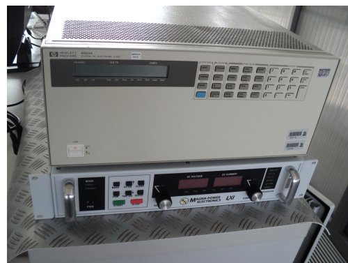
Fig. 9. Front panels of the fuel cell emulator Magna Power Electronics and the programmable electronic load HP 6050A.
