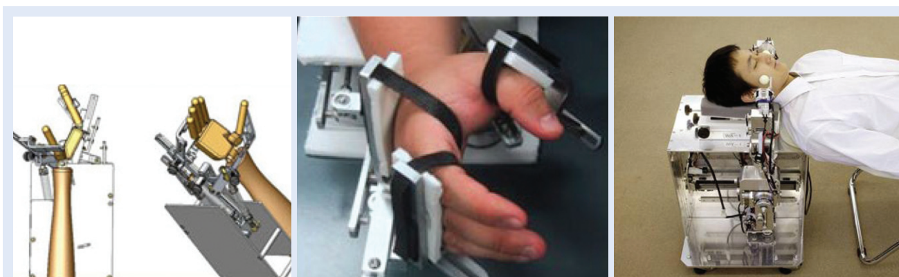
Slika 4. Robotska šaka za rehabilitaciju i robot za masažu WAO-1 4 Figure 4 Robotic hand for rehabilitation and massage robot WAO-1 4
