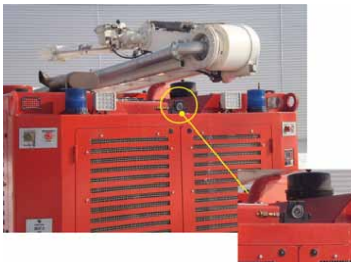
Figure 7. Cameras mounted on the front side vehicle
