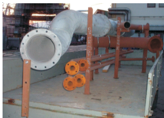
Slika 1. Primjer CAD modela sklopa cjevovoda i gotov sklop spreman za ugradnju na brod [3] Figure 1 Example of the CAD model piping assembly and of an assembly ready for installation on board a ship [3]
