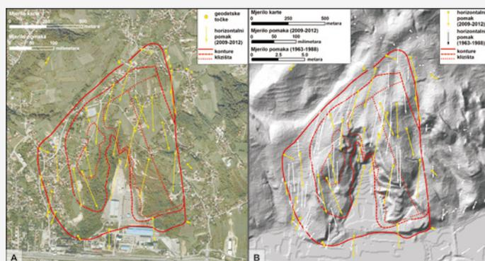
Slika 2.4.a Horizontal movement of landslide Kostanjek in period from 2009. to 2012.; Figure 2.4b Comparison of horizontal movements between epoch 2009.-2012. and epoch 1963.-1988
