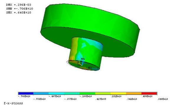
Figure 12. The stress distribution of welding pin for copper welding.
