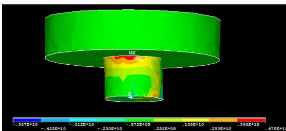
Figure 10. Stress distribution of welding pin at 20 s with 1200 rpm and 60 mm/min.
