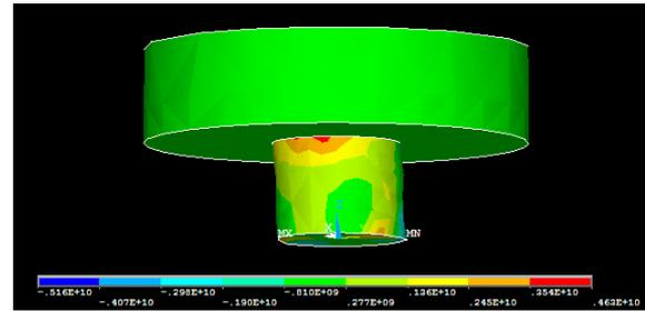
Figure 11. The stress distribution of welding pin at 20 s with 1200 rpm and 36 mm/min.
