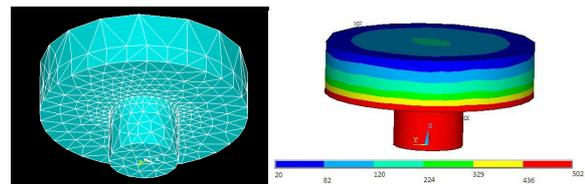
Figure 8. Mesh and temperature distribution of the welding pin.
