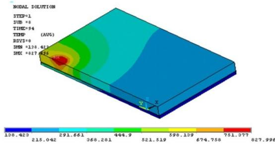
Figure 7. Temperature distribution of welded copper plate.
