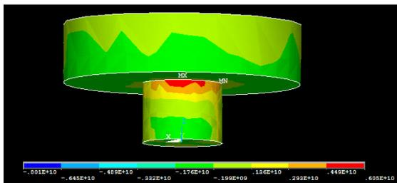
Figure 9. The stress distribution of welding pin at 4 s with 1200 rpm and 60 mm/min.
