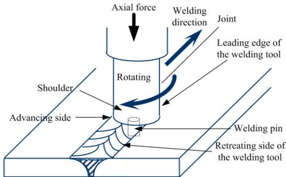
Figure 1. A schematic diagram of friction stir welding.
