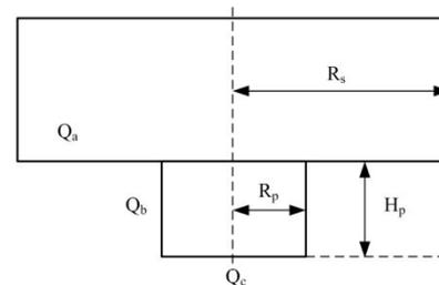
Figure 2. Shape of a welding pin.
