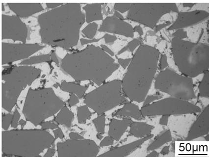
Figure 1. The original structure of Al-MMCs.
