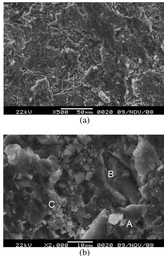
Figure 5. Fracture appearance on both sides of the composite (a) under low magnification view; (b) under high magnification view.
