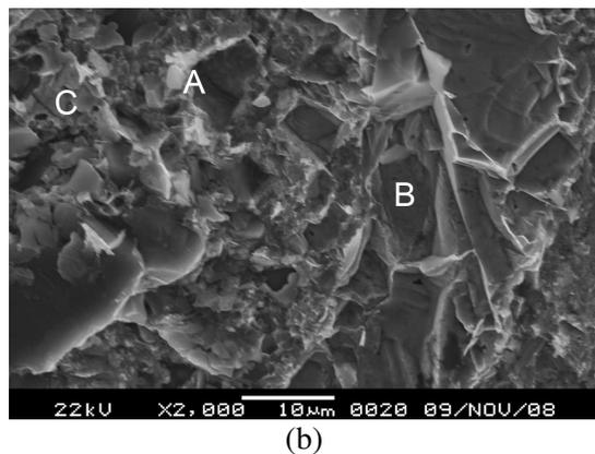
Figure 6. Fracture appearance on the side of filler metal (a) under low magnification view; (b) under high magnification view.
