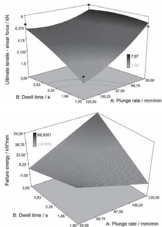
Figure 5 The influence of welding parameters on a) ultimate tensile shear force and b) failure energy
