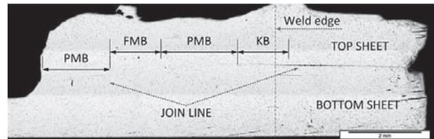
Figure 4 Macrosection and weld bond line with (FSSW at 3 000 rpm, 50 mm/min, 3 s)
