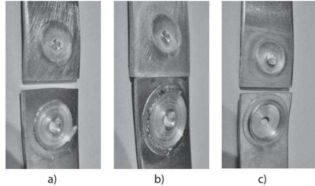
Figure 3 Examples of failure mode of samples FSSW at 2 250 rpm and a) 87,5 mm/min, 1 s; b) 87,5 mm/min, 2,25 s; and c) 24,4 mm/min, 2,25 s
