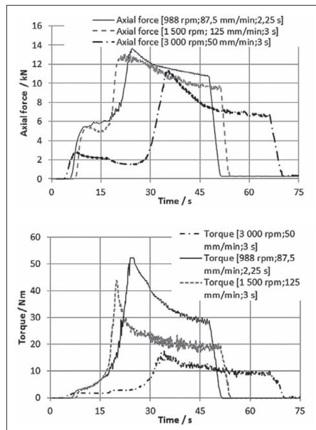
Figure 1 a) Axial force and b) torque measured with dynamometer during FSSW
