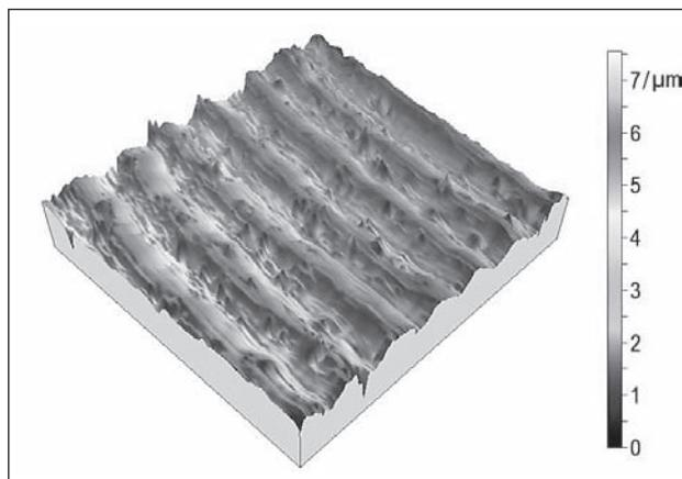
**Figure 7** Surface topography at different magnifications generated with  $v_c = 400$  m/min,  $f = 0,08$  mm/rev and  $r_s = 0,8$  mm.  $Sa = 0,49$  μm,  $Sz = 13,2$  μm,  $Sp = 5,43$  μm,  $Sku = 7,82$ ,  $Ssk = -0,67$
