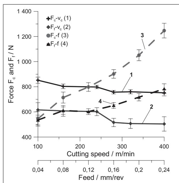
Figure 2 Influence of cutting speed and feed rate on  $F_c$  and  $F_f$  forces
