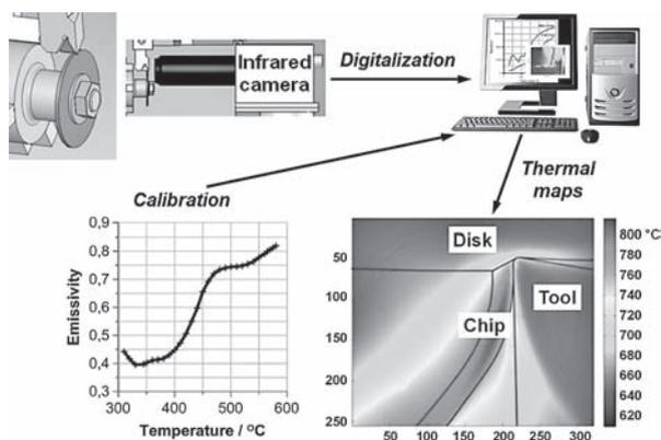
Figure 1 Scheme of IR thermal mapping technique
