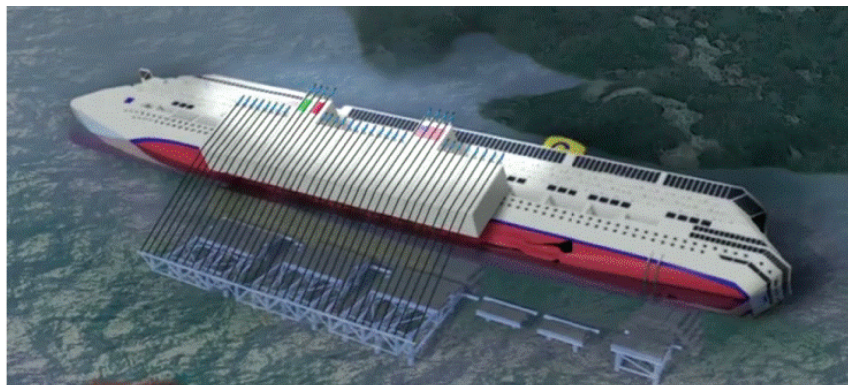
Slika 6. Omatanja brodskog trupa užadi Figure 6 Ship's hull wrapping with ropes
