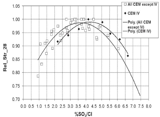
Fig. 4 – Relative 28 days strength as function of %SO<sub>3</sub>/CL
