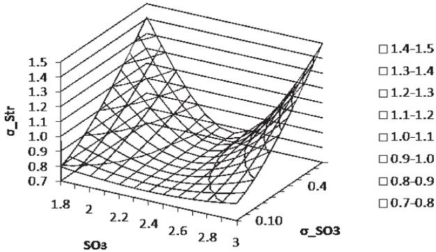
Fig. 15 – Strength 28 days standard deviation as function of %SO<sub>3</sub> content and standard deviation for CEM II B-M (P-L) 32.5
