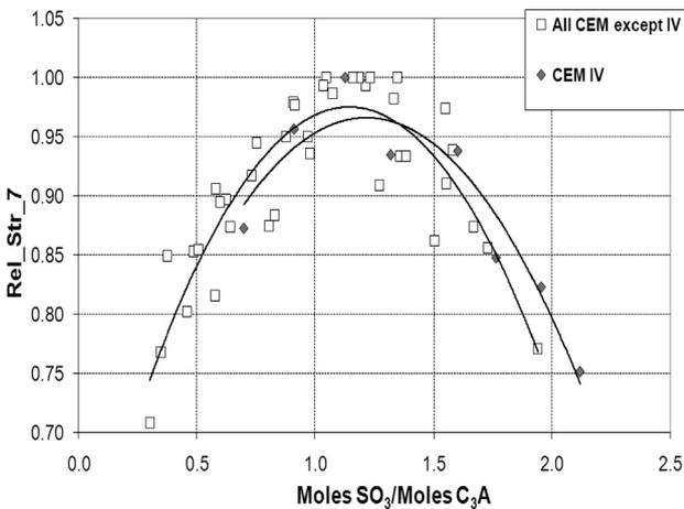
Fig. 5 – Relative 7 days strength as function of Moles SO<sub>3</sub>/Moles C<sub>3</sub>A
