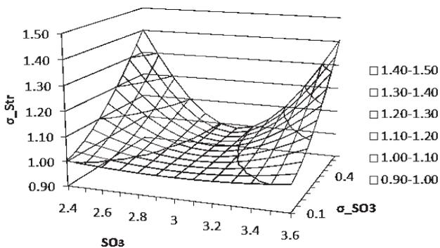
Fig. 16 – Strength 28 days standard deviation as function of %SO<sub>3</sub> content and standard deviation for CEM II A-L 42.5
