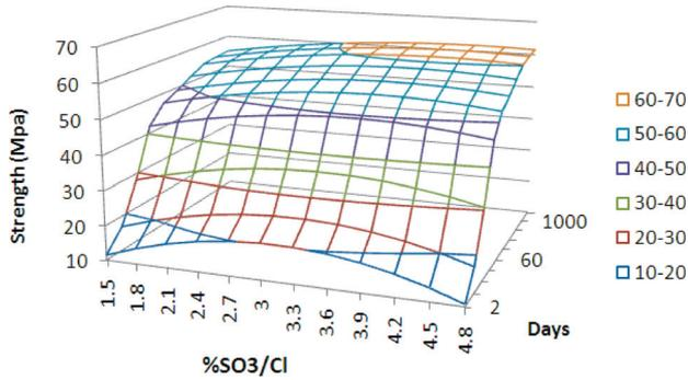
Fig. 13 – Compressive strength as function of %SO<sub>3</sub>/Cl and time
