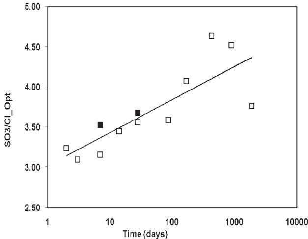
Fig. 8 – Optimum  $SO_3/Cl$  as function of curing time
