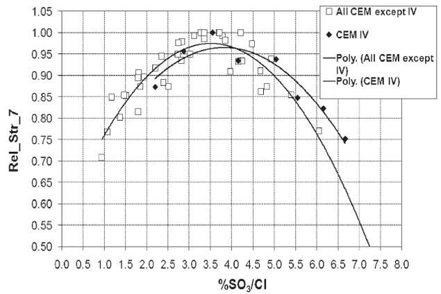
Fig. 3 – Relative 7 days strength as function of %SO<sub>3</sub>/CL
