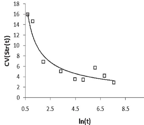
Fig. 9 – CV of strength as function of curing time
