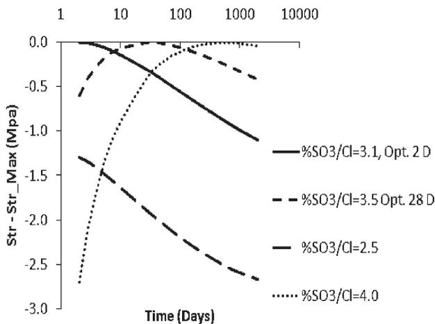
Fig. 14 – Difference strength – strength<sub>Max</sub> as function of %SO<sub>3</sub>/Cl and time
