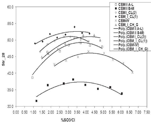
Fig. 2 – Function between Str28 and %SO<sub>3</sub>/CL
