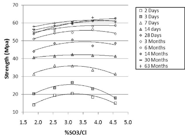
Fig. 7 – Strength as function of %SO<sub>3</sub>/Cl and age
