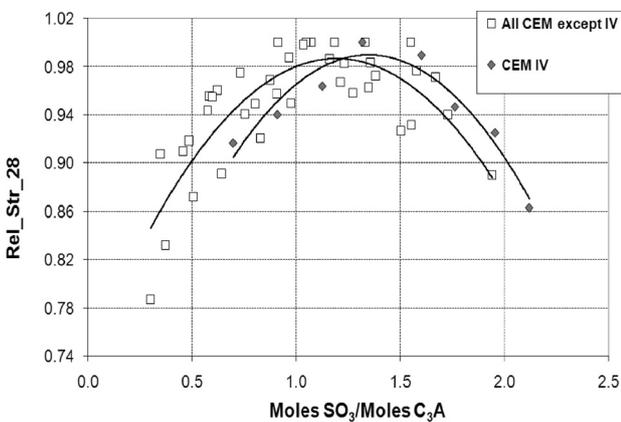
Fig. 6 – Relative 28 days strength as function of Moles SO<sub>3</sub>/Moles C<sub>3</sub>A
