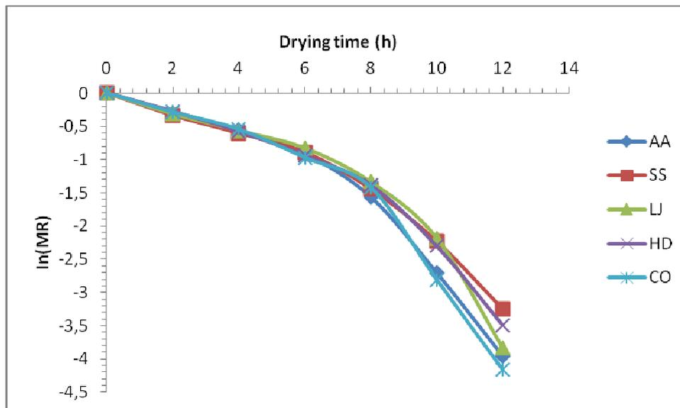
Fig. 2. Variation in  $\ln(MR)$  with time for the untreated(control) mango slices
