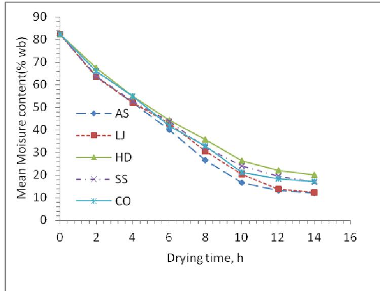
**Fig. 1.** Variations of moisture content versus drying time for the control and various pretreated mango slices
