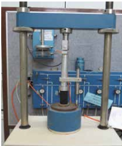
Figure 3. Uniaxial compression test using 5kN load frame
