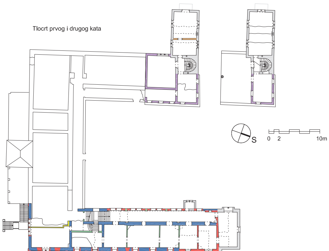
2. b, c. Građevni razvoj dvorca, prizemlje i prvi kat (dokumentacija HRZ-a, izradili P. Puhmajer, M. Bogadi) Construction development of Opeka castle, ground floor and first floor (Croatian Conservation Institute documentation, drawing by P. Puhmajer, M. Bogadi)
