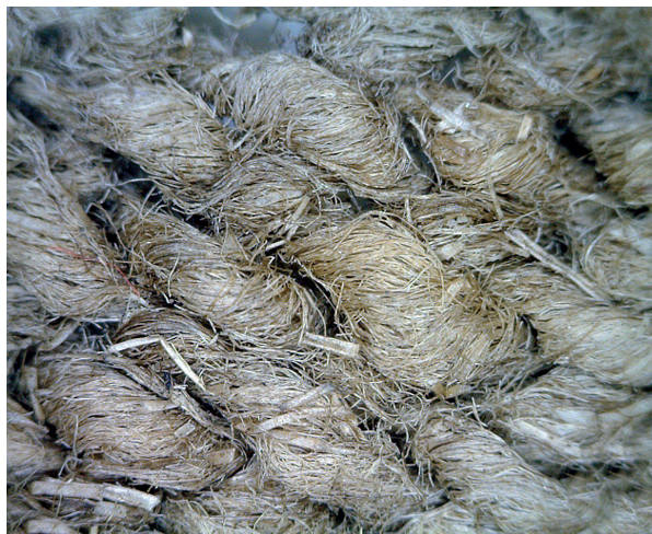
9b. Mikroskopski snimak (60 x) uzorka nakon uklanjanja konsolidanta (fototeka HRZ-a, snimila K. Hrepić) Microscopic image (60x) of the sample after removing the consolidant (Croatian Conservation Institute Photo Archive, photo by K. Hrepić)
