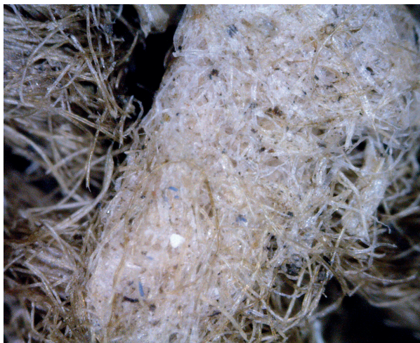
9a. Mikroskopski snimak (201 x) uzorka sa zatečenim konsolidantom (fototeka HRZ-a, snimila K. Hrepić) Microscopic image (201x) of the sample with pre-existing consolidant (Croatian Conservation Institute Photo Archive, photo by K. Hrepić)
