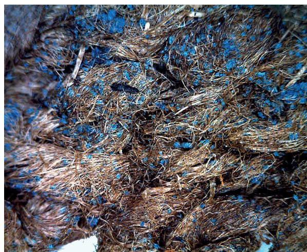
9c. Mikroskopski snimak (58 x) uzorka sa vivijanitom (fototeka HRZ-a, snimila K. Hrepić) Microscopic image (58x) of the sample with vivianite (Croatian Conservation Institute Photo Archive, photo by K. Hrepić)
