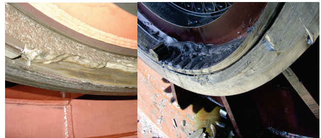
Figure 3 Failure of external bearing ring and pitting dust collected by oil flow
