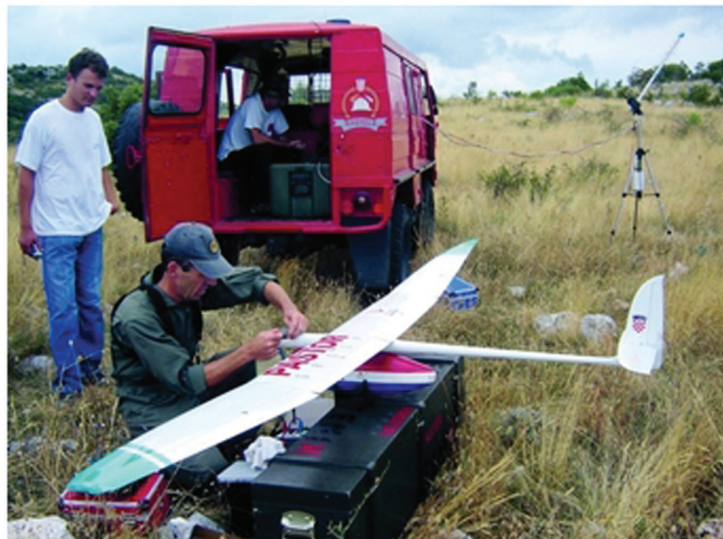
Figure 9. Croatian unmanned aerial vehicle Fenix (Cvitić, 2007)
