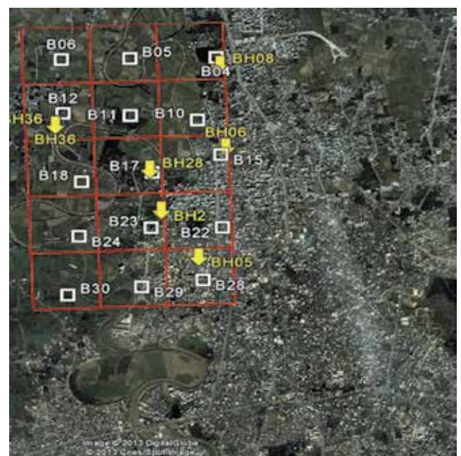
Figure 4. Location of microtremor recordings station and geotechnical boreholes
