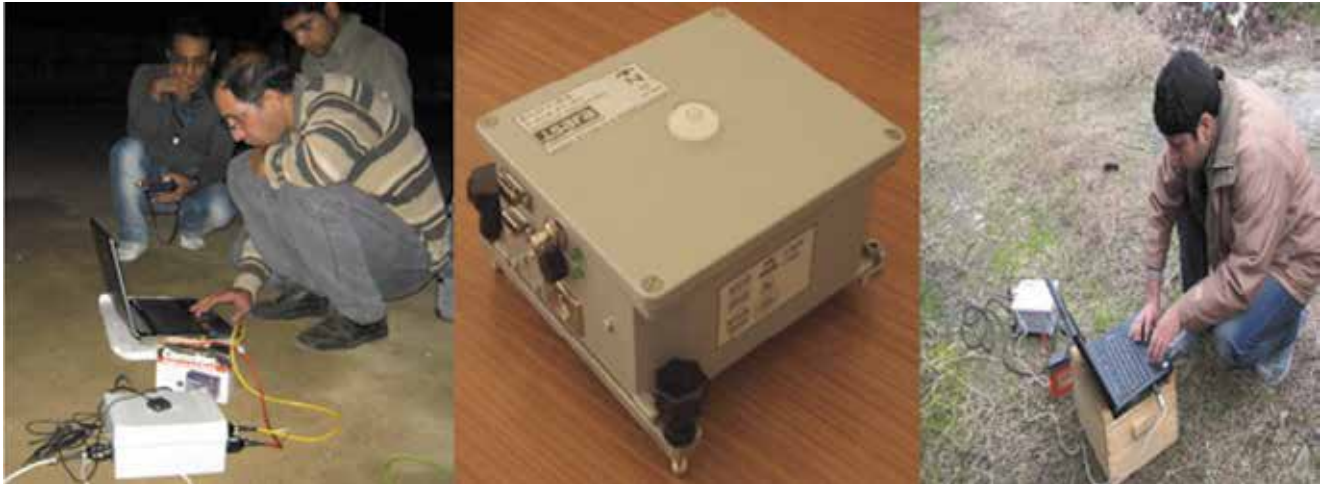
Figure 5. Microtremor observation and instrument set-up for microtremor measurements
