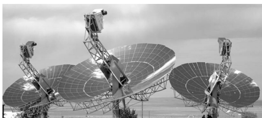
Figure 2. Dish-Stirling system. SES (Stirling Energy Systems) prototype .
