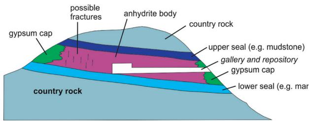
**Figure 2.** A sulphate body as a repository for low-/intermediate level radioactive waste.
