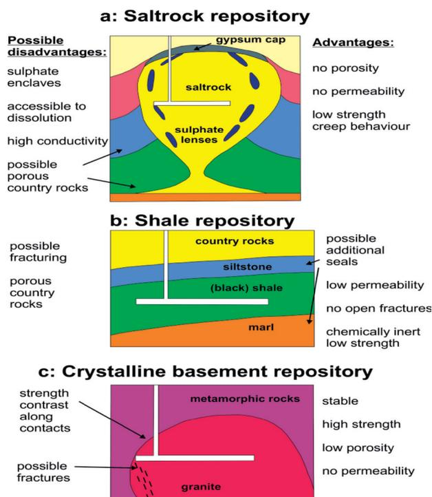
**Figure 1.** Overview on underground geological storage of radioactive waste. a – Salt diapirs. b – Silty to clayey shale/slate (phyllite). c – Crystalline rocks.
