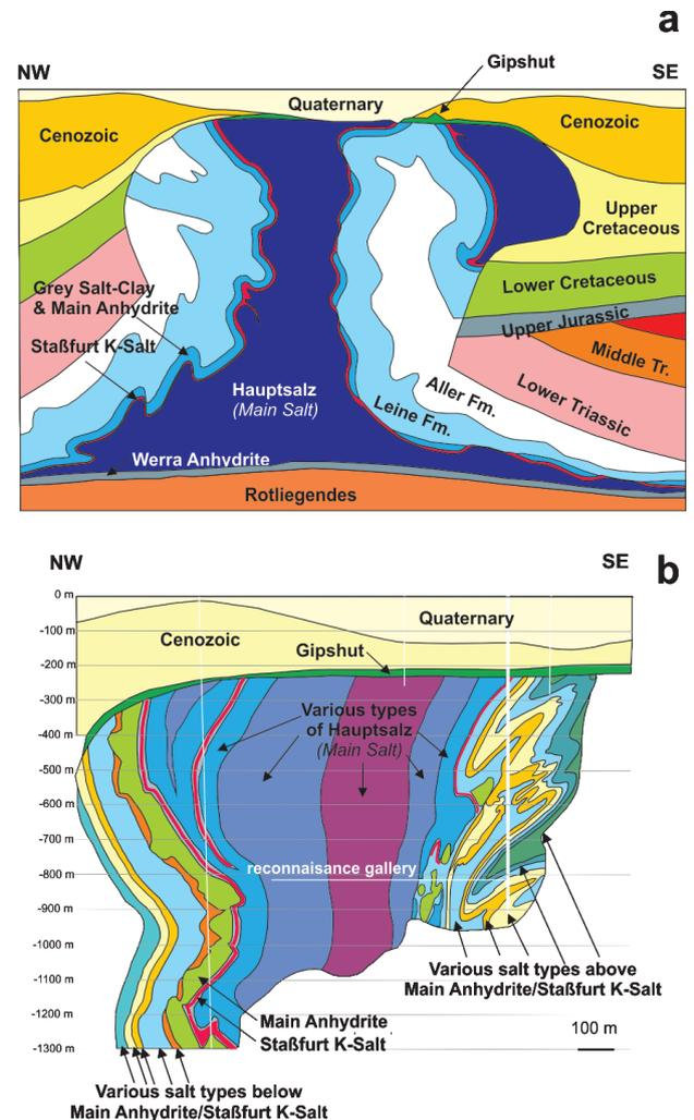
**Figure 3.** The Gorleben example (Germany) as a radioactive waste repository. a – At depth, a partly hypothetical section showing welding of feeding Zechstein stratum. b – Cross-section at the repository level (from [www.endlagerung.de](http://www.endlagerung.de) finally accessed February 25, 2012).
