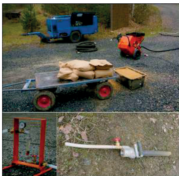
Figure 3 Up: Spraying set, Down: water flow regulator and spraying nozzle.
