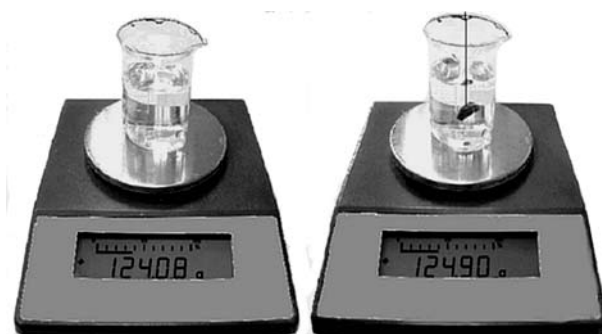
Fig. 1. Immersion method. A jar with distilled water was placed on the scale and weighed (left). Then, the kidney suspended by a thin thread was immersed in the jar so that it was fully covered by water and did not touch the bottom of the jar (right). The new weight in grams minus the weight of the jar and water divided by the specific gravity of distilled water ( \sim 1.0 ) was the volume of the kidney in cubic centimeters ( 124.90 - 124.08 = 0.82/1 = 820 \text{ mm}^3 ).
