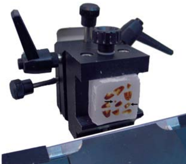
Fig. 3. Blocking and sectioning of the slabs using a microtome. The selected slabs, the punched circle (right arrow) and the slab which the circle was punched out from (left arrow).
