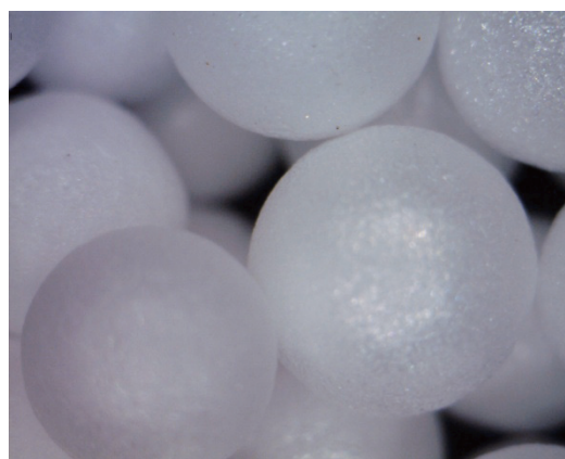
Slika 2. Zrnca granuliranog EPS-a (1,5 mm - 3,5 mm, 50×) Figure 2. Grains of granulated EPS-a (1,5 mm - 3,5 mm, 50×)
