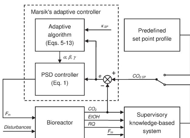
Fig. 1 – Overall scheme of the adaptive control
