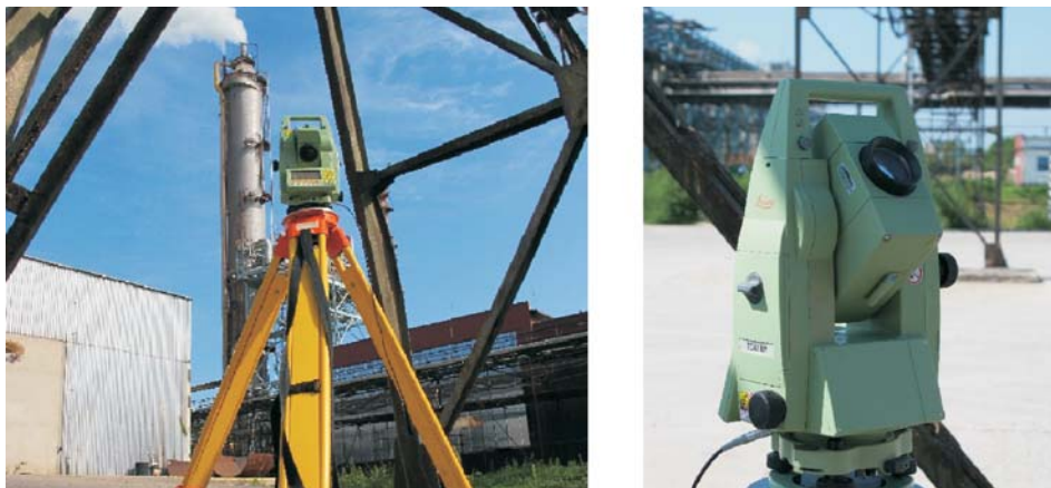
Fig. 2. The Leica TCRA1101 robotic station.
