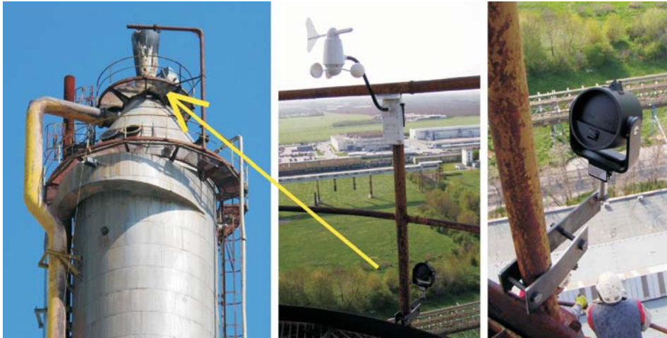
Fig. 5. The prism and Nexus meteorological station on the top of the tower.
