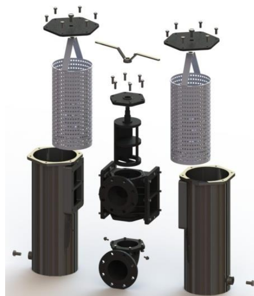
Figure 9. 3D model of a dual oil and fuel filter – exploded view
