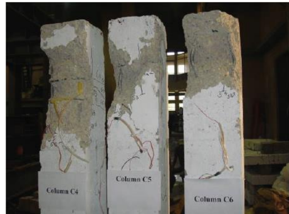
Figure 4. Characteristic damage of columns subjected to axial force (J. Němeček et al.)
