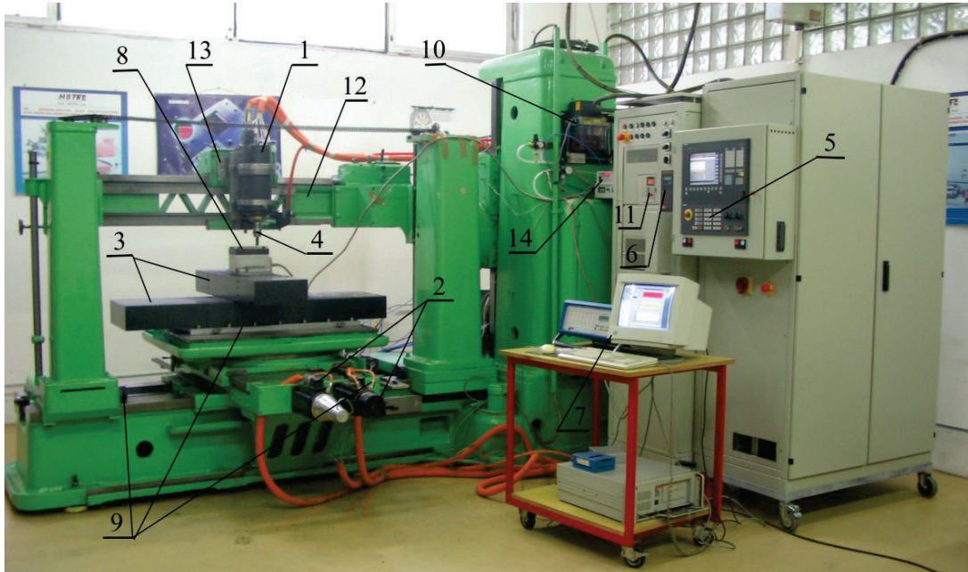
Figure 1 Machining system VBS (1 - HSM motor spindle, 2 - Electromechanical driving system, 3 - Direct driving system by linear motors, 4 - System tool – tool interface, 5 - Control unit SINUMERIK 840D, 6 - Control unit CLM 01, 7 - Equipment for measuring of cutting forces, 8 - Workpiece, 9 - Safety system, 10 - Lubrication system of motor spindle –Vogel, 11 - Frequency regulator of motor spindle Yaskawa, 12 - Bracket arm, 13 - Motor spindle carrier, 14 - Cooling control of motor spindle and linear motors)
