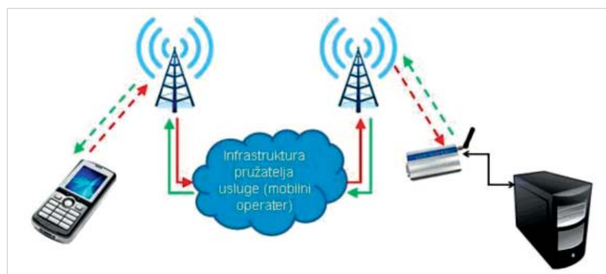
Slika 3. Prijenos SMS poruke preko GSM modemskeg sklopa Picture 3 The text message transmission via GSM modem complex
